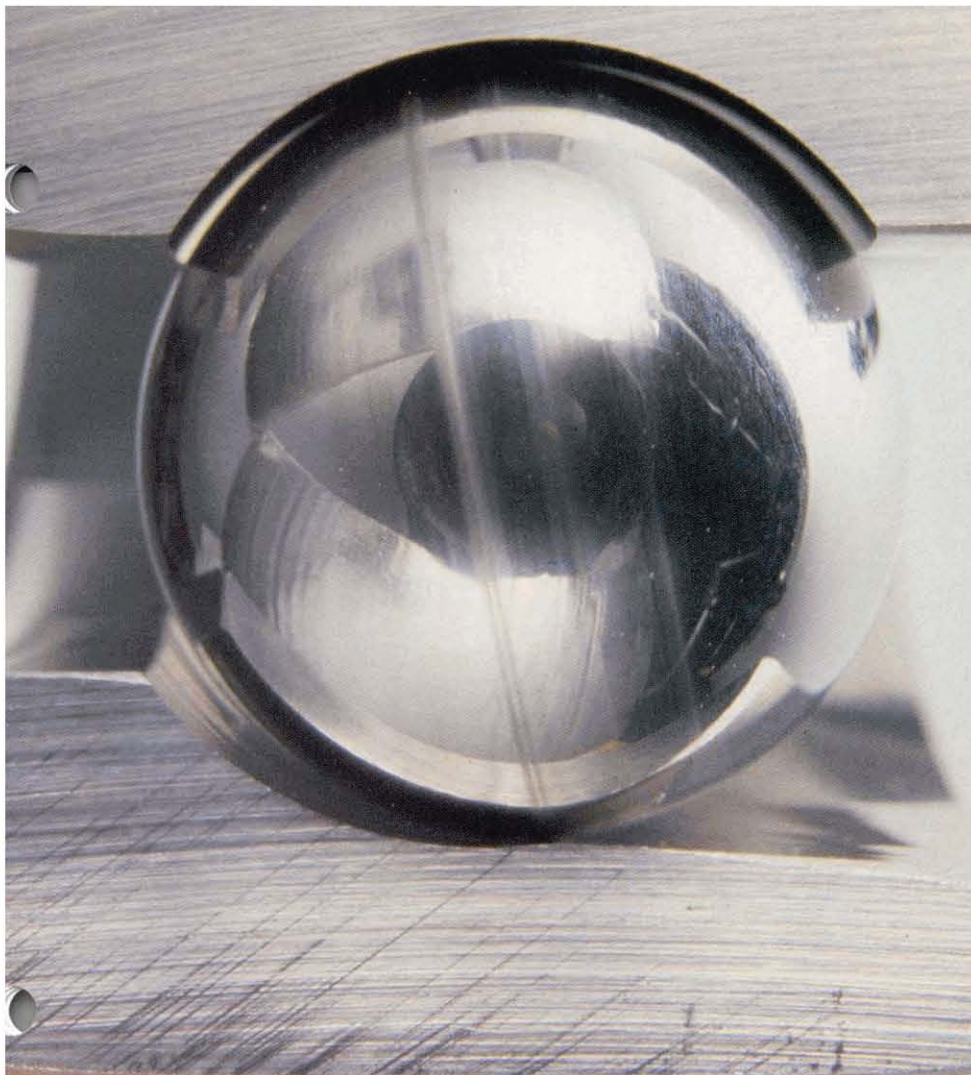
Thrust load applied to wrong faces results in wear band on balls.
